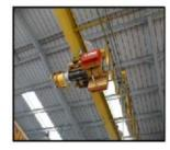
Trolley Mounted Overhead Hoists
