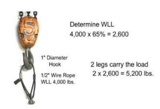
wire rope around an object, or double our wire rope slings, this D/d ratio must be calculated. For D/d ratios that fall between the values shown, use the lower efficiency.
