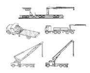
Booms and Mounts: Category 4 cranes have different types of boom configurations such as: telescoping, non-telescoping, and articulating. They may be mounted on flatbed trucks, trailers, stake beds, rail cars, barges and pontoons, or may be stationary mounted on piers, wharves, and docks.
