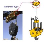
hoist upper-limit switches. A spring-loaded switch opens the circuit when the hook block raises the weight. Interruption of power to the hoist function stops the upward movement of the hoist block to prevent two-blocking.
