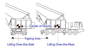
same load applied, whenever the center of gravity of the crane moves closer to the tipping axis. This is why most mobile cranes have a higher over-the-rear capacity than over-the-side.
