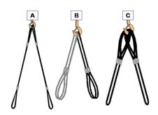
wires may become permanently deformed or bent. If a sling is doubled to the point where it is permanently set, it should not be used in a vertical or straightened out configuration because straightening the sling could cause the wires strands to break.
