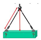
(Sling Length + Height) X Weight Distribution = Sling Angle Stress
