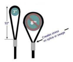
eye. If the hook diameter is too large, a shackle can be used to connect the slings to the hook, thereby reducing the diameter over which the sling eyes are placed.
