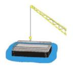
increased load on the crane and rigging gear. Tide changes and wave action can cause overloads, shock loads and loss of control. A plan should be developed to account for these.
